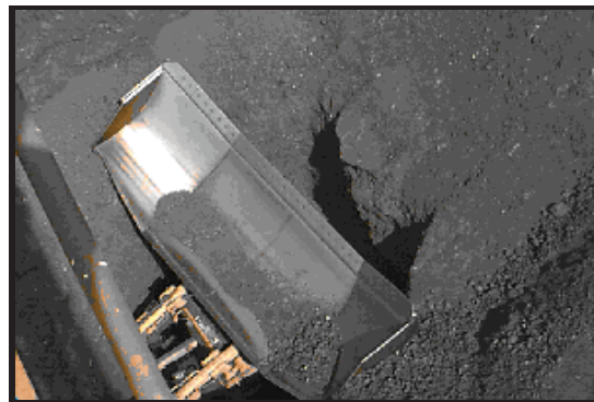
A bulldozer completely buried after falling into a feeder air cavity.
